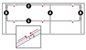
**2.** Attach one of the side frames (B) directly to the center frame (A) and the remaining side frame to the center frame.
